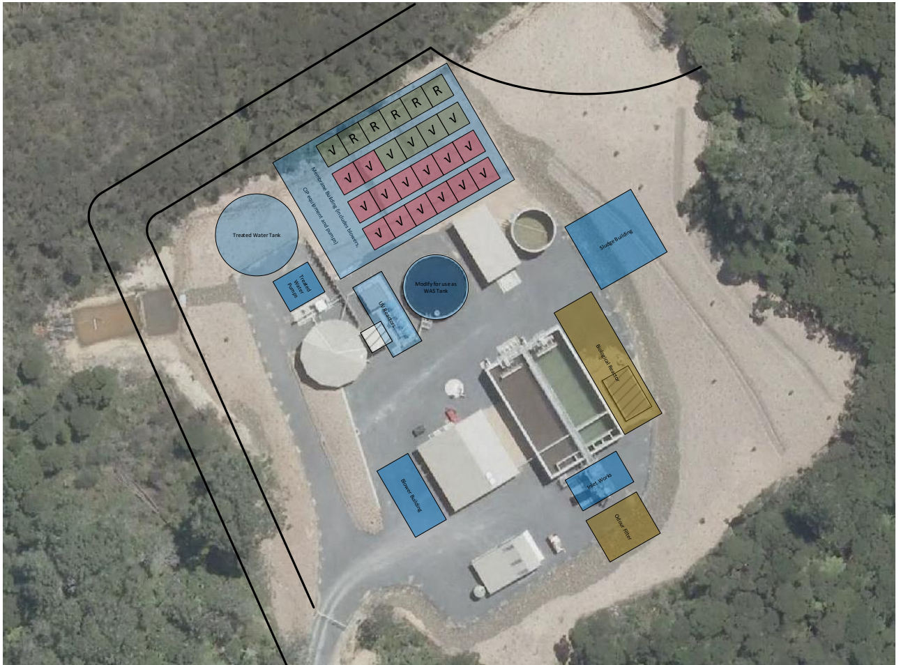
Figure 12 Proposed layout of the 7,000 connections upgrade required by 2060 or 2089, depending on the connection rate assumed. Areas in yellow indicate the additional equipment required for the 7,000 connections upgrade.
