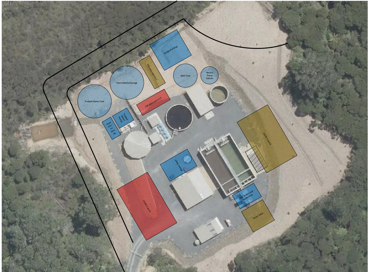
Figure 10 Proposed layout of the 7,000 connections upgrade required by 2060 or 2089, depending on the connection rate assumed. Areas in yellow indicate the additional equipment required for the 7,000 connections upgrade.
