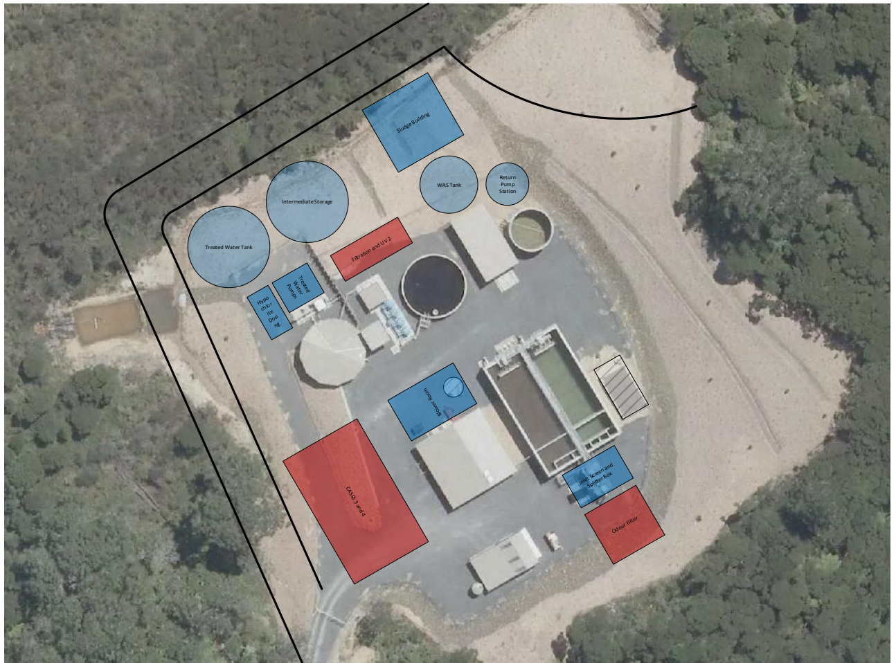
Figure 9 Proposed layout of the 5,000 connections upgrade required by 2028 or 2032, depending on the connection rate assumed. Areas in red cater for 5,000 connections only, where areas in blue allow for future staging, by allowing sufficient capacity or space for the 7,000 connections upgrade.
